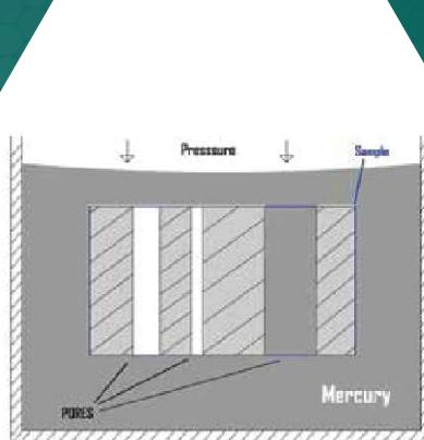
the volume of intruded nonwetting liquid are accurately measured. Combining these data with the surface tension and the contact angle of the liquid, pore diameter, pore volume, pore volume distribution and pore surface area are computed.
